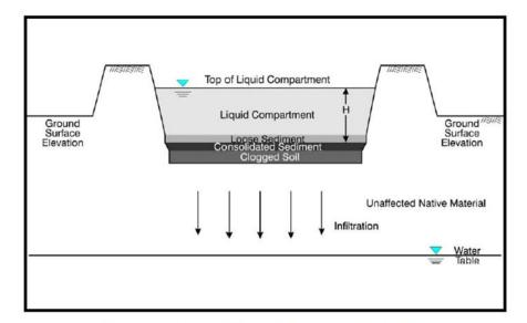
Figure 2.3 Schematic Cross-Section View of SI Unit.
